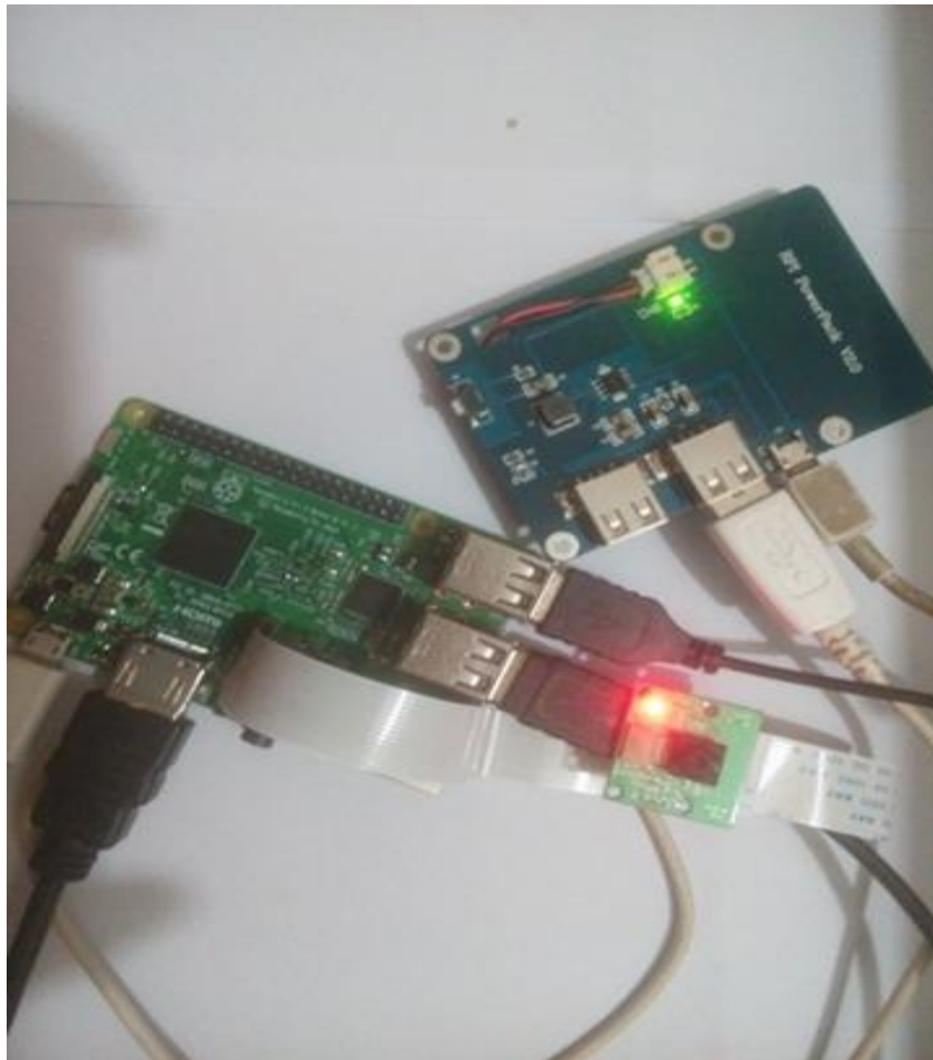
Figure 3.8: Connection raspberry pi with camera
