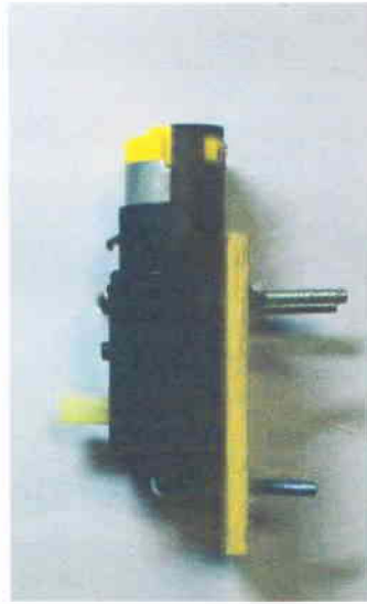
Figure 4-2: Motor attached with small pitches of hard board by screw
