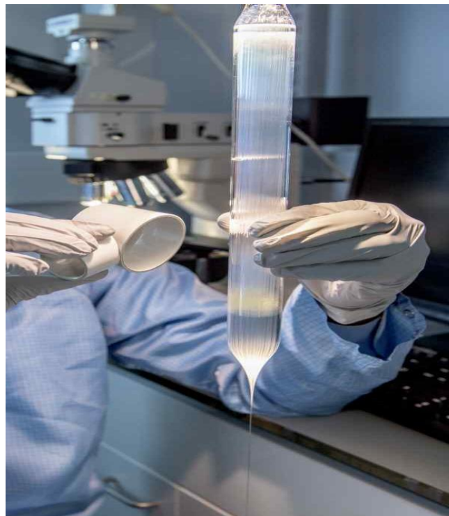
Figure 1.3: Inspection of a preform for a photonic crystal fiber
