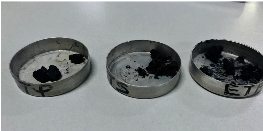
Figure 3.10: Moisture Content Measurement of Textile ETP, Tannery Sludge and Mixture of Textile ETP, Tannery Sludge
