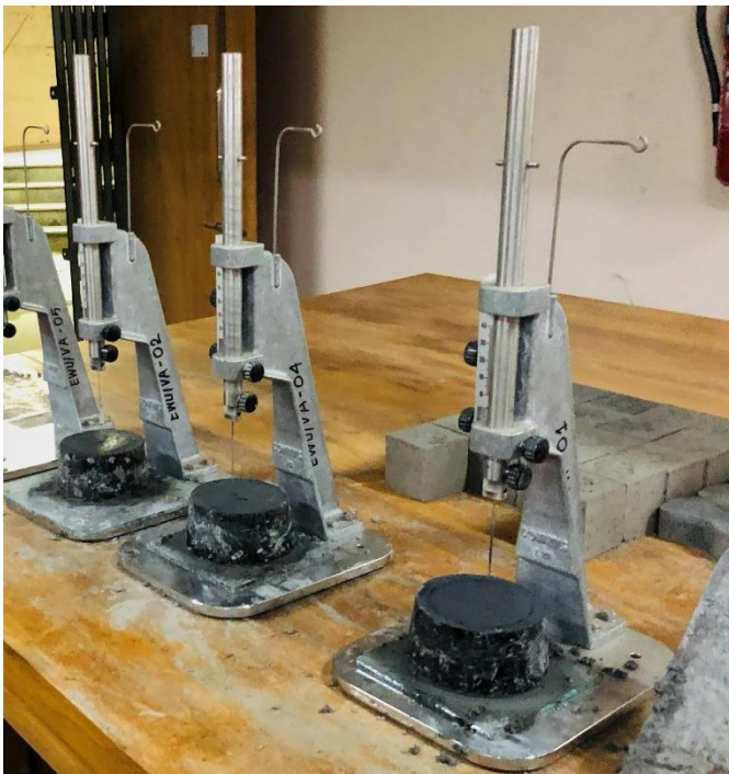
Figure 3.19: Initial and Final Setting Time Measurement of Cement Mixed with Sludge Samples by Weight
