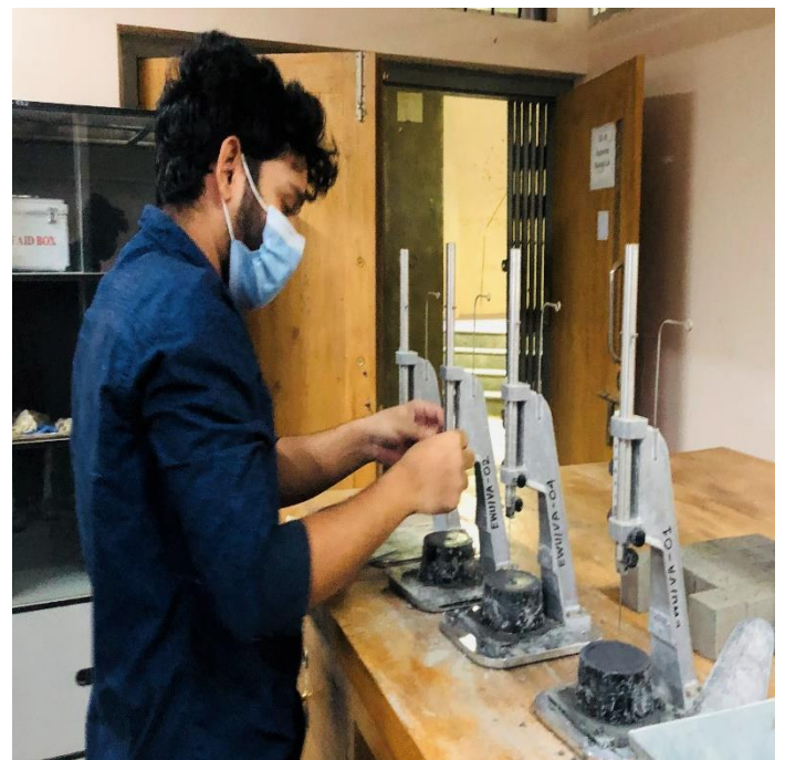
Figure 3.19: Initial and Final Setting Time Measurement of Cement Mixed with Sludge Samples by Weight
