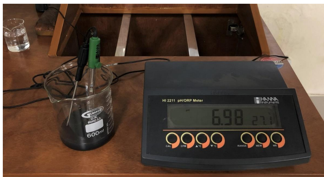
Figure 3.14: Mixture of Tannery and Textile Effluent Treatment Plant Sludge pH Measurement
