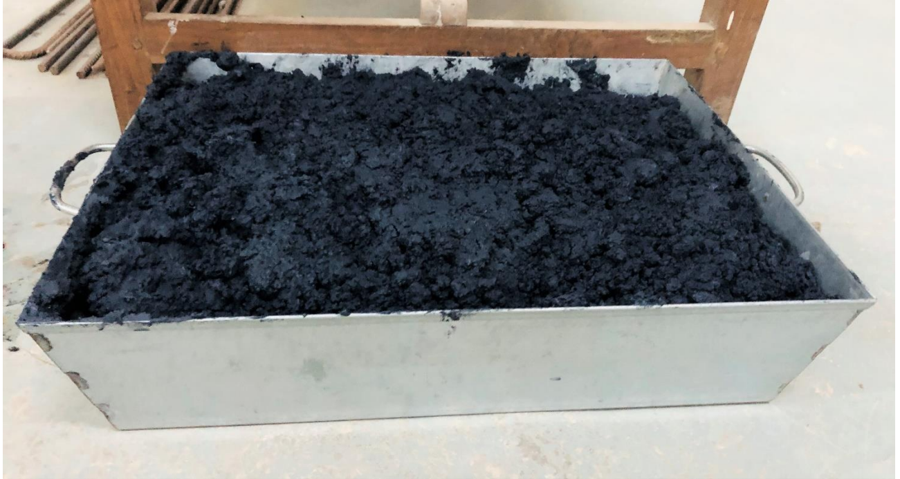
Figure 3.7: Textile Effluent Treatment Plant Sludge Before Dry Condition
