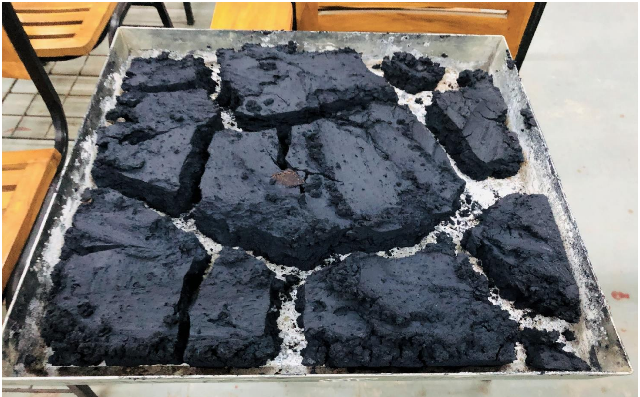
Figure 3.8: Textile Effluent Treatment Plant Sludge After Dry Condition
