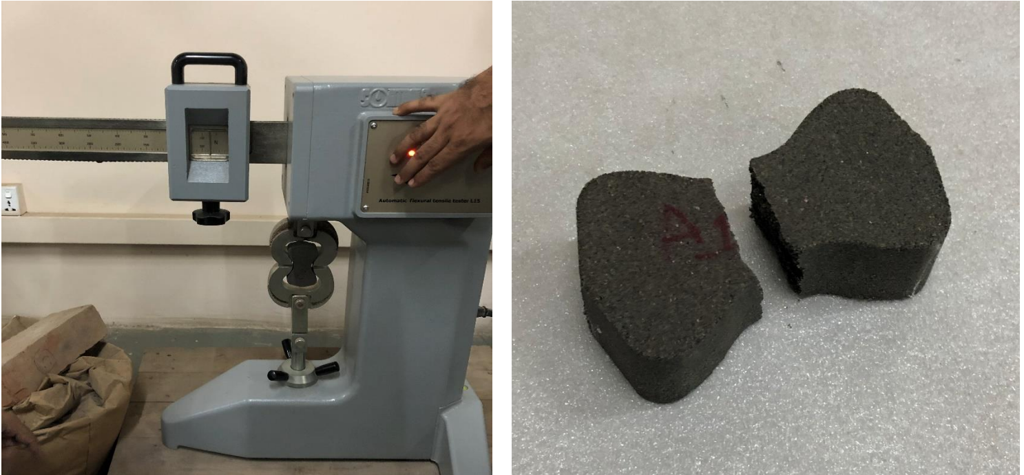
Figure 3.21: Tensile Strength of Cement Mortar Briquet
