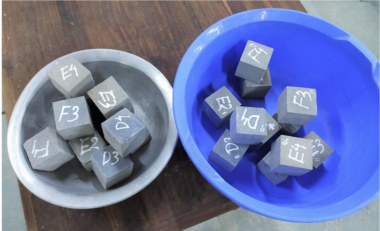
Figure 3.23: Oven Dried Cement Mortar Cubes for Water Absorption Measurement
