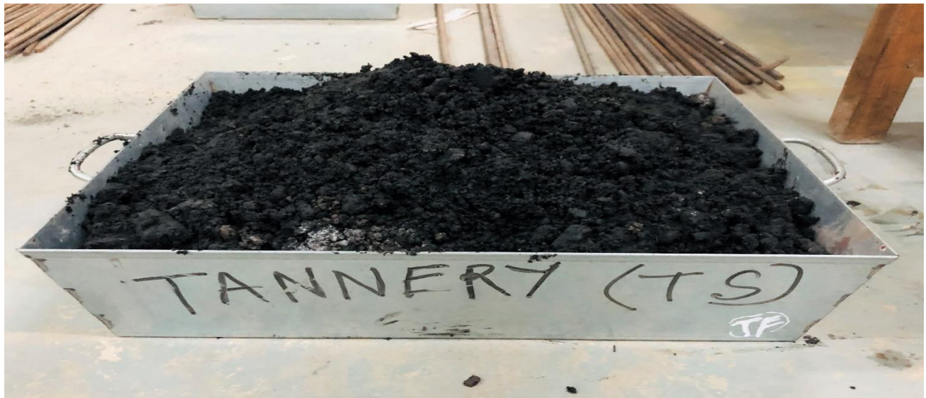
Figure 3.5: Tannery Sludge Before Oven Dry Condition
