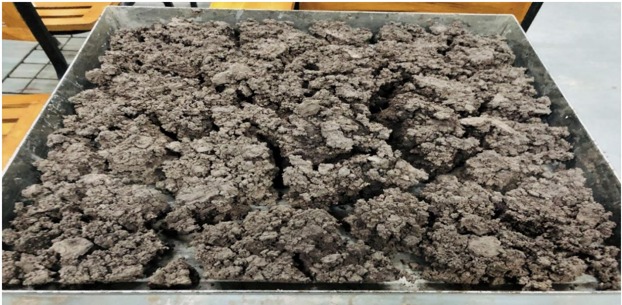
Figure 3.6: Tannery Sludge After Oven Dry Condition
