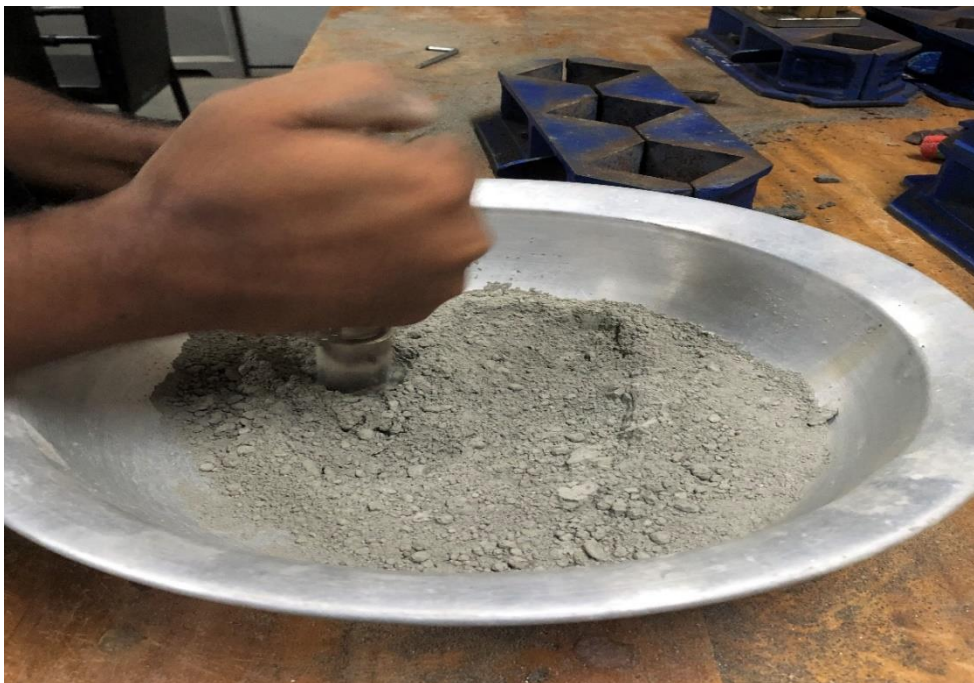
Figure 3.9: Sludge was Hammered and turned into Power Form
