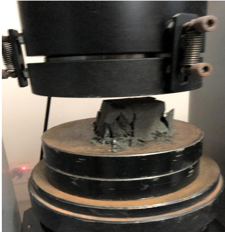
Figure 3.20: Compressive Strength of Cement Mortar Cube
