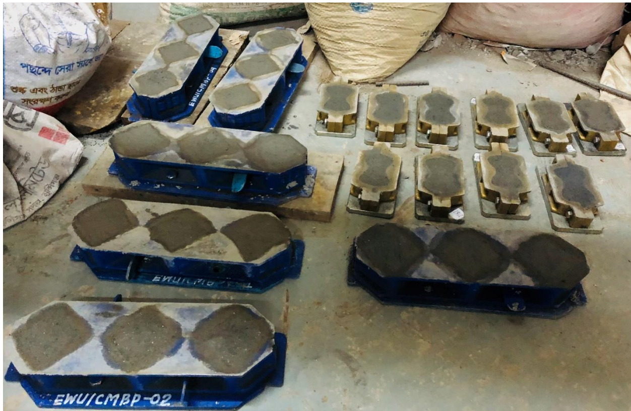
Figure 3.16: Cement Mortar Cube and Briquet was Prepared
