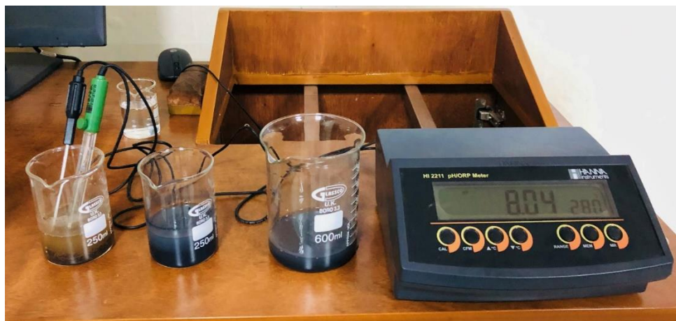
Figure 3.12: Tannery Sludge pH Measurement
