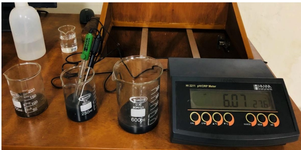
Figure 3.13: Textile Effluent Treatment Plant Sludge pH Measurement
