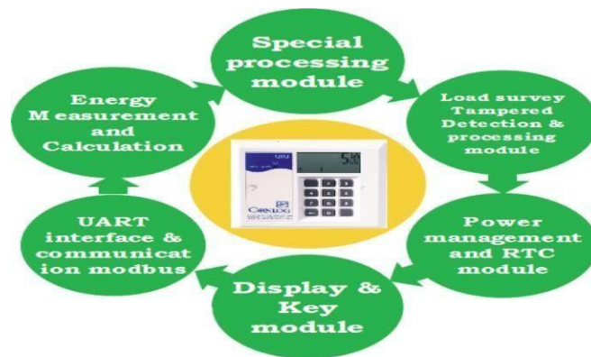
Figure-2: Software architecture of a conventional meter, showing communications with other meter components
