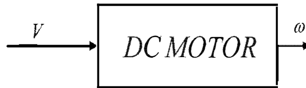
Figure 3.2: A simple open-loop System
