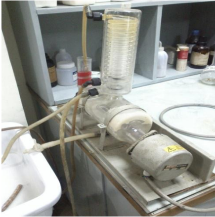
Fig 2.3: GENRISTO Distill Water Plant
