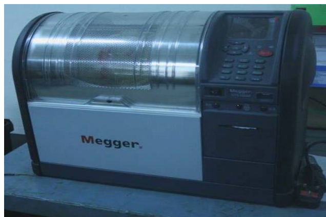
Figure 4.1: Oil testing machine-Megger OTs100F [2]
